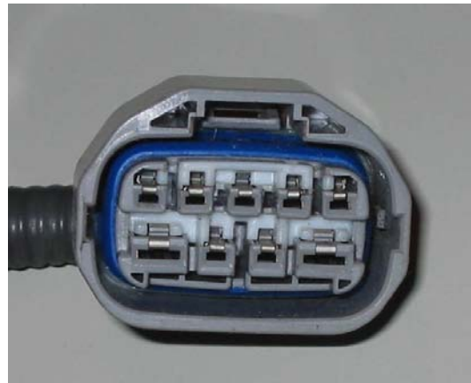
Figure 5. Toyota A650E 9pin lever position connector
