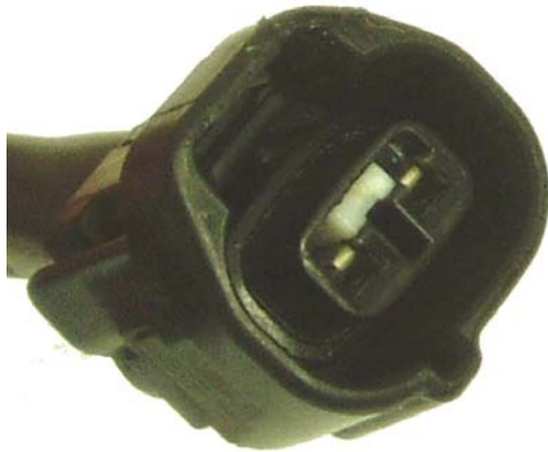
Figure 6. Toyota A650E driveshaft and torque converter speed 2-pin connectors
