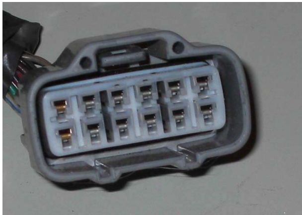
Figure 4. Toyota A650E 12-pin solenoid connector
