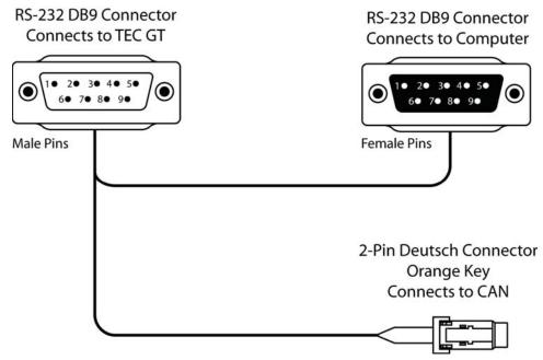
The pinout for this harness is shown in the table below. All pins not listed below are not connected on the TEC GT adapter harness.
